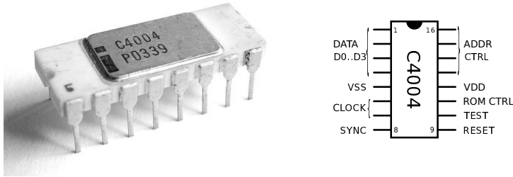
Figure 100: Left: DIL chip of an Intel 4004. (Wikipedia) Right: pin-out of chip.
