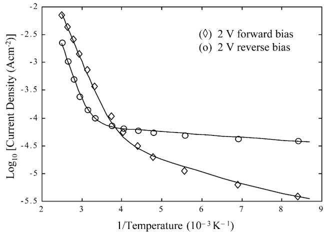
Fig. 3. Arrhenius plot of the current recorded under an applied bias of (◇) 2 V forward bias, and (○) 2 V reverse bias.
