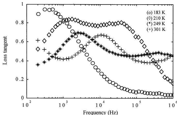
Fig. 5. The temperature dependence of loss tangent.
