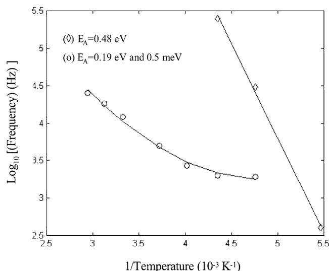
Fig. 6. Arrhenius plot of the frequency position of the peaks in the loss tangent of Fig. 5. The plot reveals an activation energy of 0.48 eV for the high frequency peak and of 0.19 eV for the low frequency peak.
