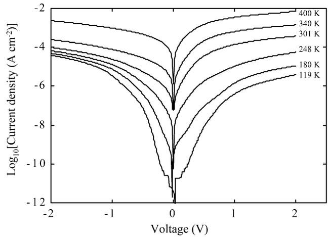
Fig. 2. Temperature dependence of the current-voltage characteristics.
