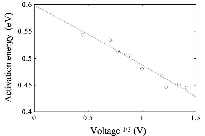
Fig. 4. Decrease of the activation energy,  $E_A$  for the reverse current vs.  $V^{1/2}$ .
