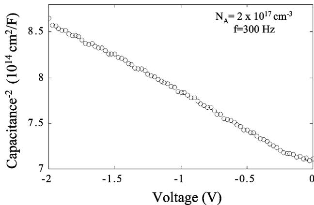
Fig. 1. Reciprocal capacitance squared vs. bias, recorded at a frequency of 300 Hz.
