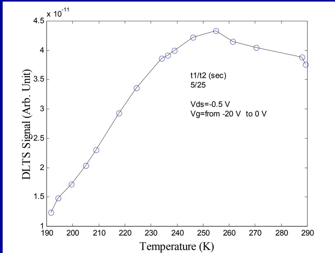
DLTS spectra of drain-current transients due to gate bias pulse from  $-20$  V to  $0$  V.
