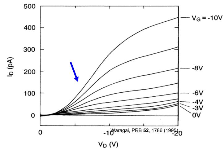
Explained by model of Poole and Frenkel. Traps!
