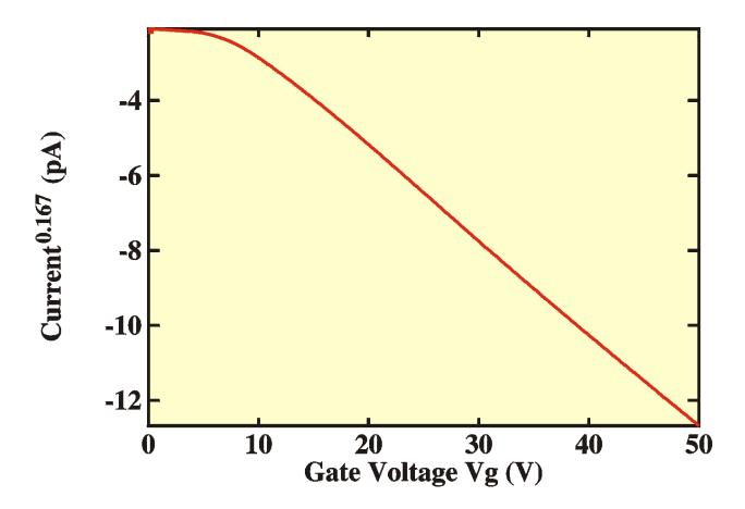
Non-linear Transfer curves explained by model of Shur and Hack for amorphous silicon. Traps!
