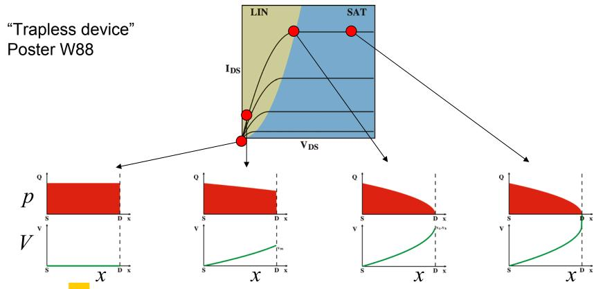
At small  $V_{\rm ds}$ , homogeneous device
