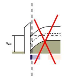
2. A TFT normally works in accumulation and thus cannot store the immobile charge needed for band bendings (there are no electronic states,  $N_A^-$ ).
