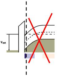
2. A TFT normally works in **accumulation** and thus cannot store the immobile charge needed for band bendings (there are no electronic states,  $N_{\rm A}^{-}$ ).
