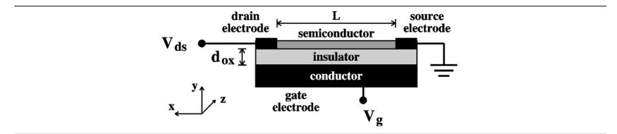
2: At any place in the device, the current is proportional to the local field and charge density:
