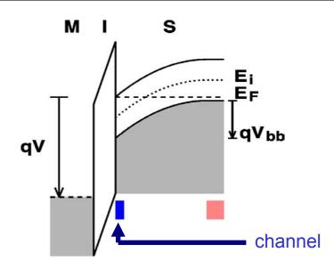
When the Fermi level at interface is resonant with conduction band, a large density of charge is induced. This is the so-called "channel"
