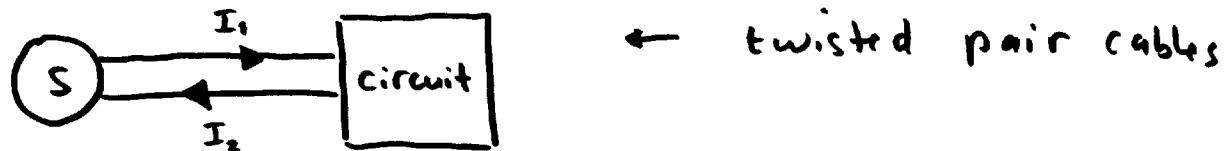
in current. One wire has positive current. The other wire has exactly opposite current. Any noise caught by one wire is also picked up by the other cable and the difference stays the same:
