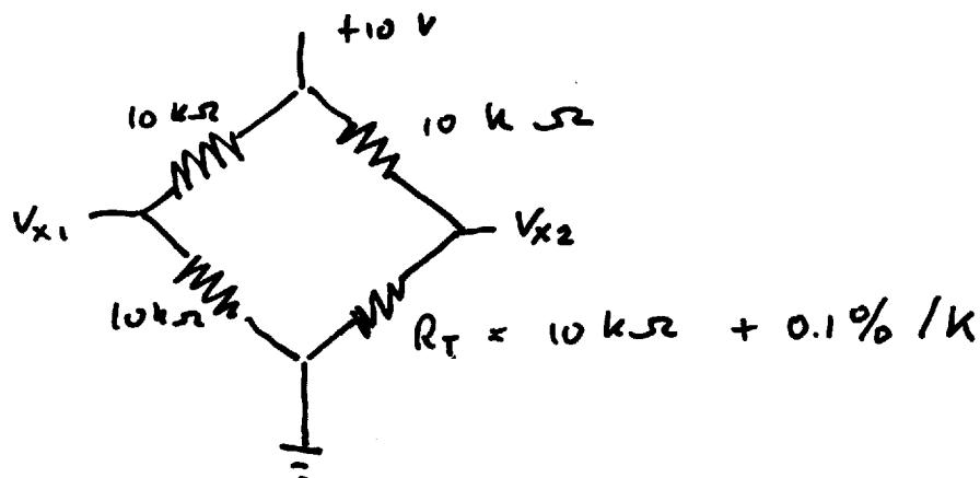
$V_{x_1}$  is always at 5 Volt.  $V_{x_2} = \frac{R_T}{R_T + R} \times 10 \text{ V} \approx 5 \text{ V}$
