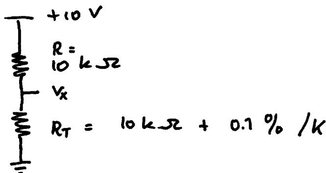
$V_x$  is around 5 volt, so we have to use the 20 volt scale of the multimeter. At that scale the voltage resolution is 10 mV. ( $= \Delta V$ ). The sensitivity is the derivative of the function  $V(T)$ .
