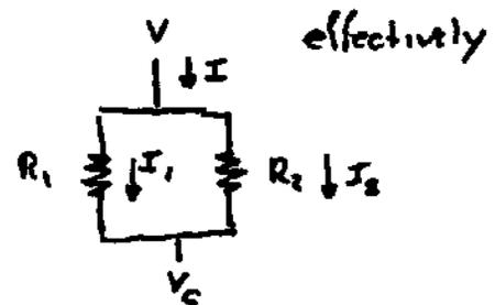
when  $V$  is changed, for instance raised, a current is drawn from  $V$  source to charge the capacitor  $C$ . This current is  $I_1$ . But a parallel current  $I_2$  is also drawn that is 'wasted'. If  $I_1 = \frac{V - V_c}{R_1}$ ,
