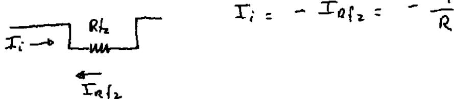
$$\text{Ohm's Law : } R_i = \frac{V_i}{I_i} = -\frac{V_i}{-V_i/R} = -R$$
