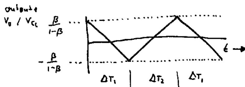
$$\text{amplitude} = \frac{\beta}{1-\beta} V_{CC}$$
