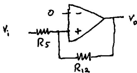
$$R_{12} = R_1 + R_2$$
