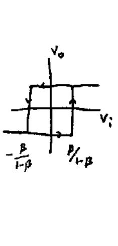
$$V_0 = -V_{cc}, \quad V_p = -V_{cc} \beta + V_i(1-\beta)$$
