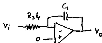
$$V_0 = -\frac{1}{R_{34} C_1} \int v_i(t) dt + V_{0g}$$
