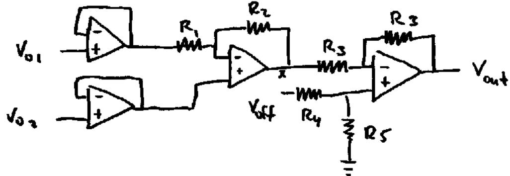
to put  $r_{in} = \infty$ ; amplifier diff.  $\rightarrow -1 \times$  amplifier plus offset ( $V_{out} = 0$ )
