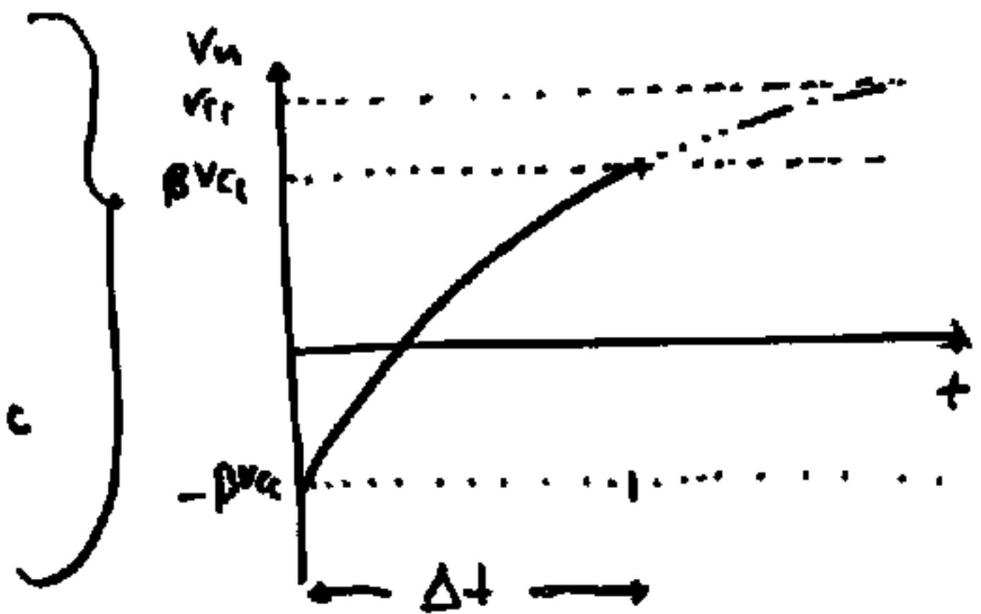
$$V_n(t) = V_{cc} - (\beta+1) V_{cc} \exp(-t/RC)$$
