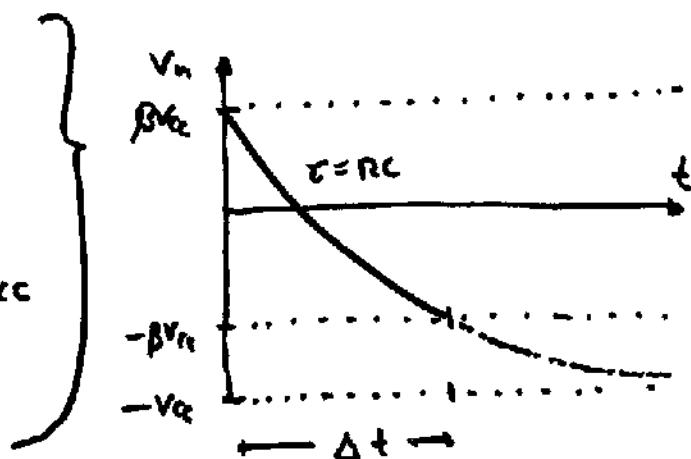
$$V_n(t) = -V_{cc} + (\beta+1)V_{cc} \exp(-t/\tau)$$
