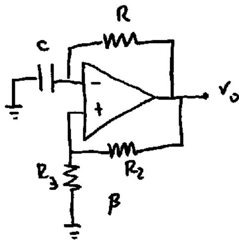
Imagine :  $V_o = +V_{cc} \Rightarrow V_p = +\beta V_{cc}$ ,  $C$  is empty  $\Rightarrow \Delta V_c = 0 \Rightarrow V_n = 0 \Rightarrow \Delta V_R = V_{cc} \Rightarrow I_R = \frac{+V_{cc}}{R}$ . This charges
