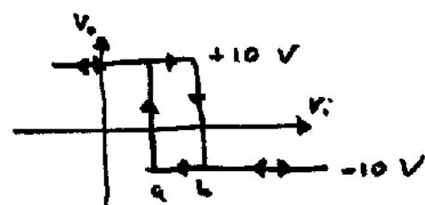
a) Type I. because for  $V_i = -\infty$ ;  $V_o = +V_{cc}$
