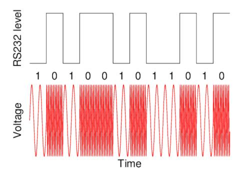
Receiver will **Dem**odulate it. 1 kHz  $\rightarrow$  1, 5 kHz  $\rightarrow$  0
