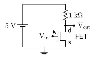
$V_{in}$  and  $V_{out}$  are relative to ground (connections similar to the 5 V power supply). Use a power FET (for example the IRF530) for this purpose. Power FET transistors normally have the connections as shown below (taken from IRF530 datasheet):
