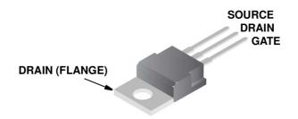
The output state is the inverse of the input state. The FET transistor works as switch. When we press the 'button' (Logical '1'; apply 5 volts at the entrance  $V_{in}$ ), the FET becomes a short circuit (R = 0) and a current flows through the resistance. This lowers the output voltage that goes to a logical '0'.
