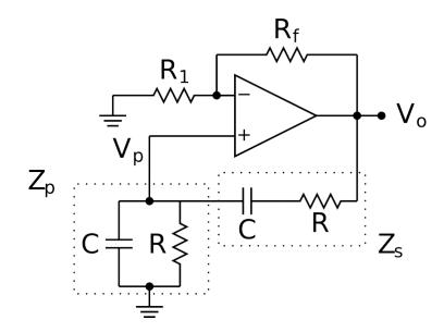
The above circuit is a Wien Oscillator. It consists of an ideal opamp with negative feedback composed of R1 and R2, and a branch with positive feedback, composed of two RC networks.
