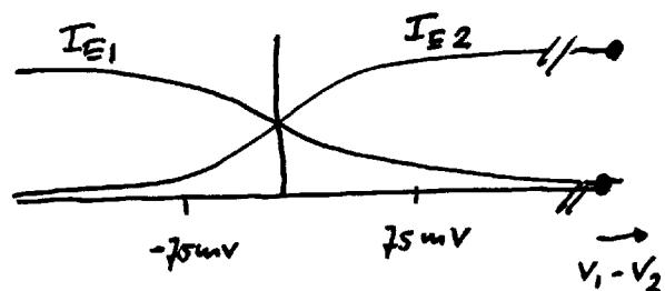
$$V_1 - V_2 = 500 \text{ mV} \rightarrow I_{E2} \approx 4.3 \text{ mA}, I_{E1} = 0$$
