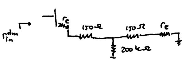
$$\begin{aligned} r_{in}^{dm} &= (\beta+1) \cdot [r_e + 150 \Omega + \\ &\quad (150 \Omega + r_e) // 200 \text{ k}\Omega] \\ &\approx (\beta+1) \cdot 2 \cdot (50 \Omega + 150 \Omega) = 40 \text{ k}\Omega \end{aligned}$$
