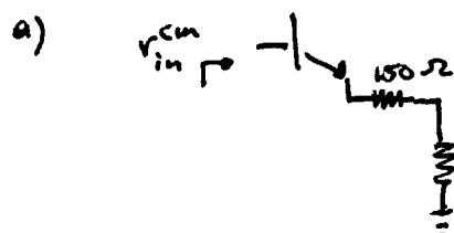
$$\begin{aligned} r_{in}^{cm} &= (\beta+1) \cdot [r_e + 150 \Omega \\ &\quad + 400 \text{ k}\Omega] \\ &\approx 40 \text{ M}\Omega \end{aligned}$$
