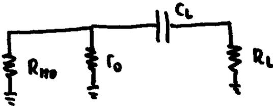
$$\begin{aligned} \tau_L &= C_L (R_{M0} // r_o + R_L) \\ &= 5 \mu\text{F} (9514 \Omega // 10 \text{ k}\Omega + 1500 \Omega) \\ &= 31.9 \text{ ms} \end{aligned}$$
