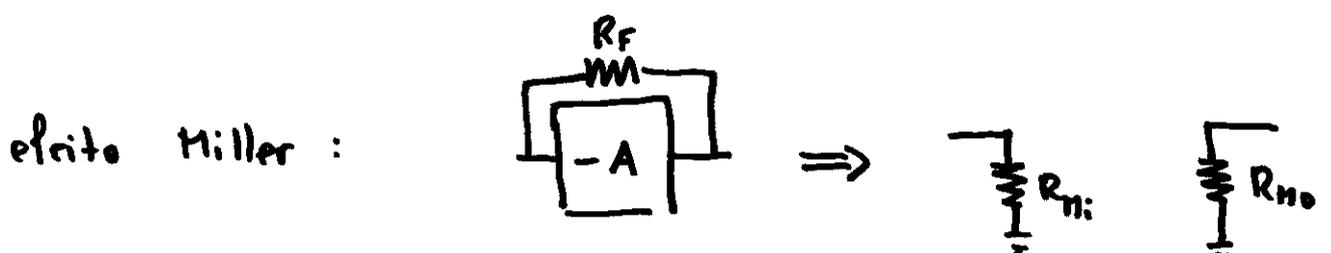
$$A = -19.565, R_{ni} = \frac{R_F}{1 - A} = 10 \text{ k} \Omega / 20.565 = 486.3 \Omega$$
