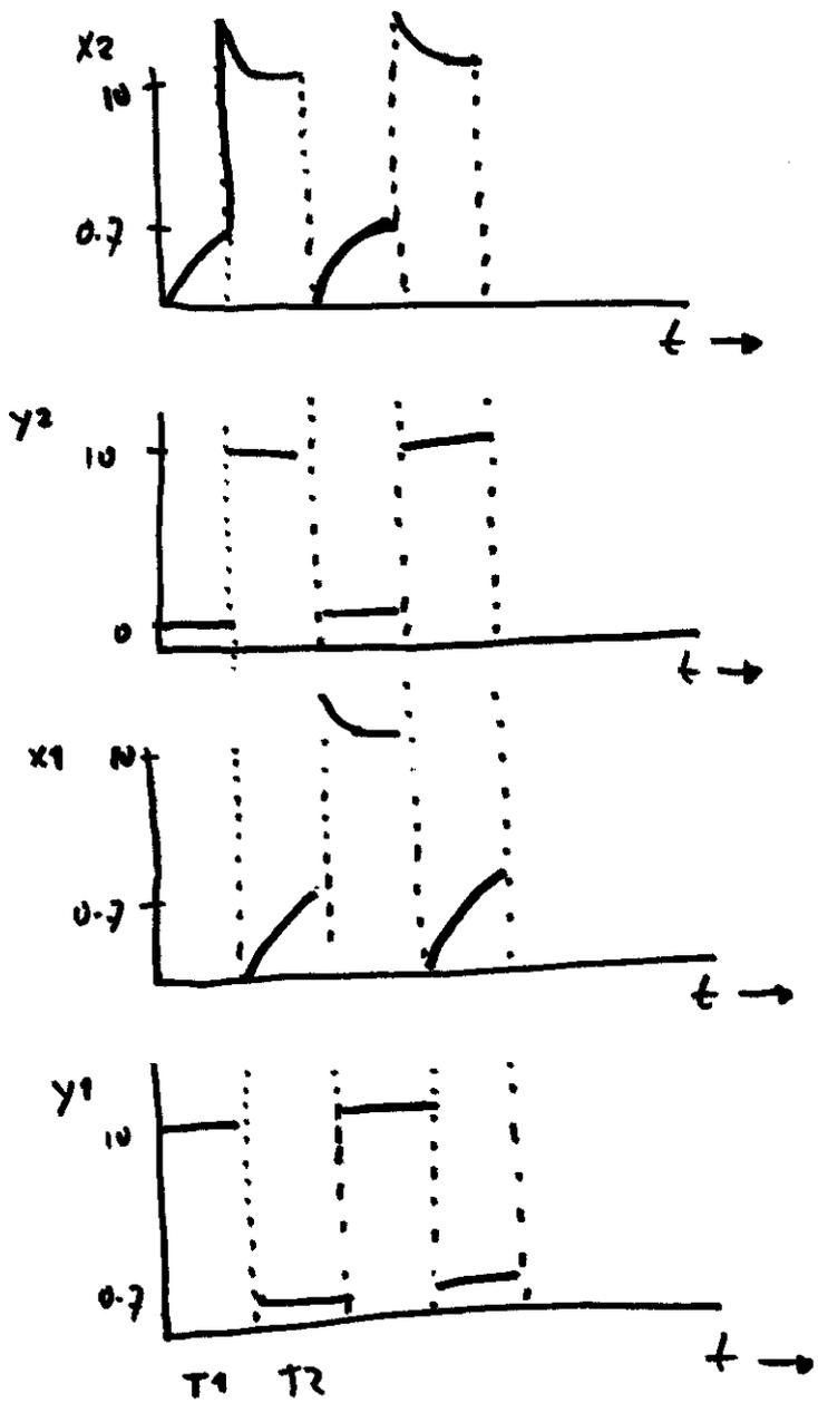
b)  $T_1 : V_{x2} = 10 (1 - \exp(-t/\tau)) = 0.7$
