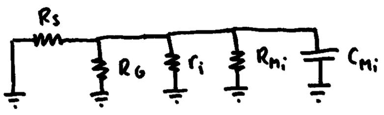
$$\tau_i = C_{mi} (R_s \parallel R_G \parallel r_i \parallel R_{mi})$$
