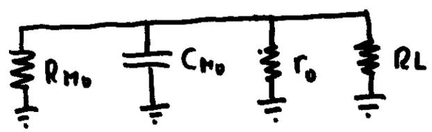
$$\tau_o = C_{mo} (R_{mo} \parallel r_o \parallel R_L)$$
