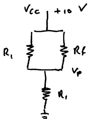
$$V_p = \frac{R_1}{R_1 + R_1//RF} V_{cc} = \frac{R_1 + RF}{R_1 + 2RF} V_{cc}$$
