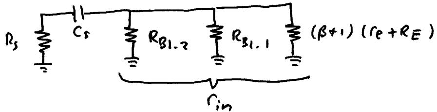
$$\tau_s = C_s R_{eff} = 10 \mu F \times 2.92 \text{ k}\Omega = 29.2 \text{ ms}$$
