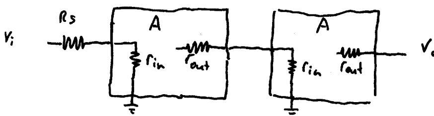
$$\frac{v_o}{v_i} = \frac{r_{in}}{r_{in} + R_s} \times A \times \frac{r_{in}}{r_{out} + r_{in}} \times A$$
