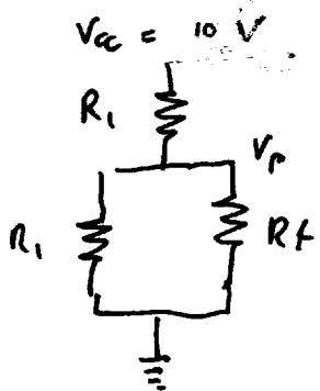
$$V_p = \frac{R_1//RF}{R_1 + R_1//RF} = \frac{RF}{R_1 + 2RF} V_{cc}$$
