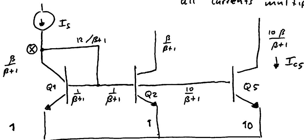
$$I_{in} \text{ at } \otimes : I_s = \frac{\beta}{\beta+1} + \frac{12}{\beta+1} = \frac{\beta+12}{\beta+1} \times I_{E1} \quad (I_{E1} = \frac{\beta+1}{\beta+12} I_s)$$
