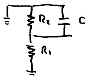
$$\frac{1}{2\pi C(R_1/R_2)} \approx \frac{1}{2\pi R_1 C}$$
