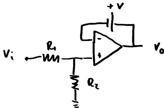
$$V_p = \frac{R_2}{R_1 + R_2} V_i \quad , \text{ amplop ideal : } V_n = V_p :$$
