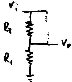
$$\frac{V_0}{V_i} = \frac{R_1}{R+R_1} = \frac{0.1}{10.1} \approx 0$$
