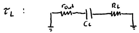
$$\tau_L = (R_L + r_{out}) C_L = (1 \text{ k}\Omega + 1 \text{ k}\Omega) \times 10 \mu\text{F} = 20 \text{ ms}, \quad f_L = \frac{1}{2\pi\tau_L} = 7.96 \text{ Hz}$$
