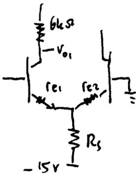
$$\frac{V_{o1}}{V_{i1}} = - \frac{R_c}{r_{e1} + r_{e2} // R_s} \approx - \frac{R_c}{2r_e} = \frac{6 \text{ k}\Omega}{50 \Omega}$$
