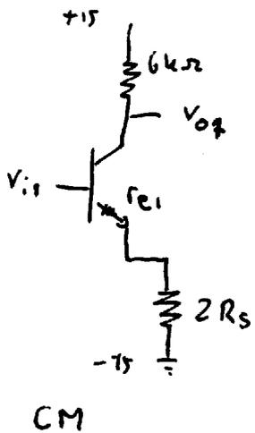
$$\frac{V_{o1}}{V_{i1}} = - \frac{R_c}{r_e + 2R_s}$$
