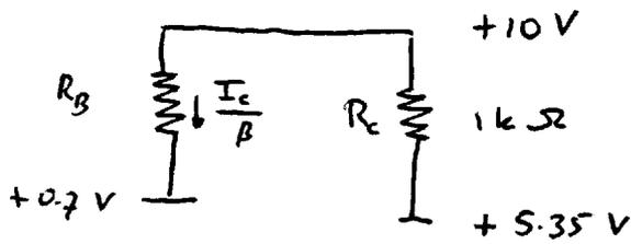
$$I_c = \frac{(10\text{ V} - 5.35\text{ V})}{1\text{ k}\Omega} = 4.65\text{ mA}$$
