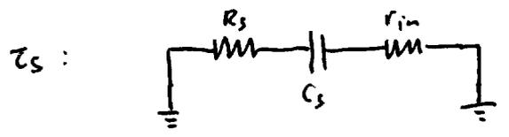
$$\tau_s = (R_s + r_{in}) C_s = (1 \text{ k}\Omega + 5 \text{ k}\Omega) \times 10 \mu\text{F} = 60 \text{ ms}, \quad f_s = \frac{1}{2\pi\tau_s} = 2.65 \text{ Hz}$$
