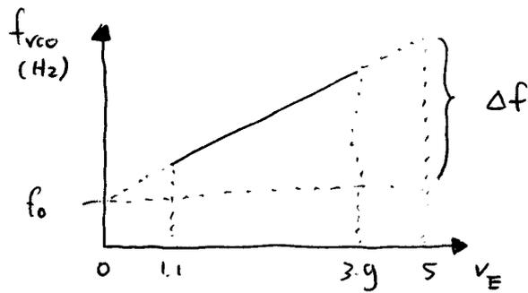
$$f_0 = \frac{1}{2\pi R_b C} \quad , \quad \Delta f = \frac{1}{2\pi R_a C}$$
