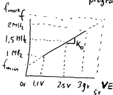
$$K_0 = \frac{df}{dV_E} = \frac{2 \text{ MHz} - 1 \text{ MHz}}{3.9 \text{ V} - 1.1 \text{ V}} = 3.57 \cdot 10^5 \text{ Hz/V}$$
