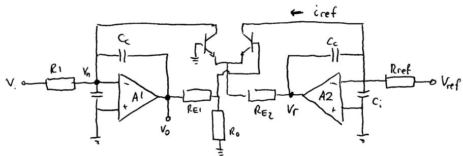
Determine the feedback ratio  $\beta = \frac{V_n}{V_0}$
