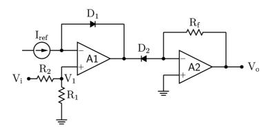
Determine the relation between  $V_{\circ}$  and  $V_{i}$ .
