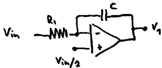
$V_n = V_p = \frac{V_{in}}{2}$ . The voltage drop over  $R_1$  is thus  $\frac{V_{in}}{2}$ .
