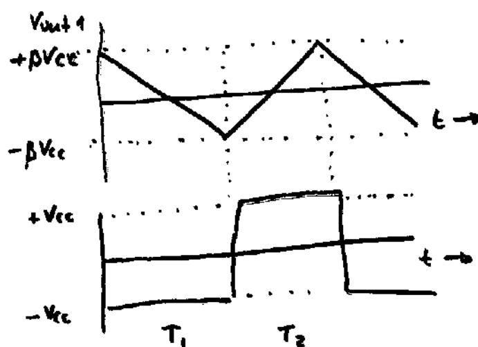
$$\text{Note: } V_{ou1} = +\beta V_{cc} \\ V_{ii} = -\beta V_{cc}$$
