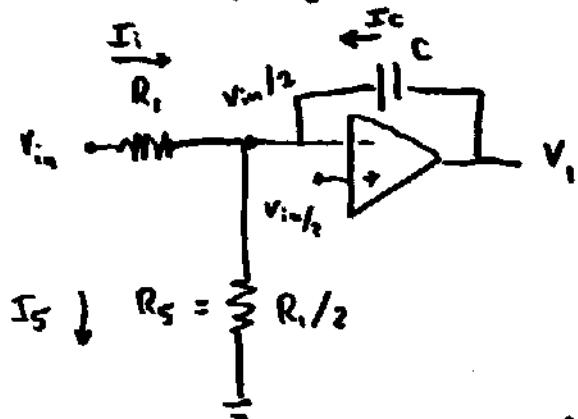
$V_n = V_p = \frac{V_{in}}{2}$ . A current flows
