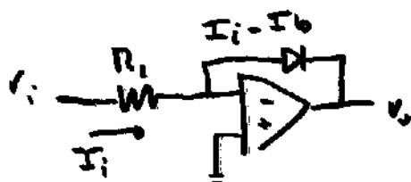
$$V_o = V_T \ln \left( \frac{V_i + I_b}{R_i} \right) / I_{S0}$$
