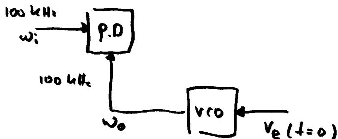
$$\text{VCO: } \omega_0 = 100 \text{ kHz} + \frac{2 \text{ kHz}}{V} \times v_e = 100 \text{ kHz}$$
