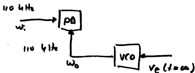
$$\omega_0 = 100 \text{ kHz} + \frac{2 \text{ kHz}}{V} \times v_e = 110 \text{ kHz}$$
