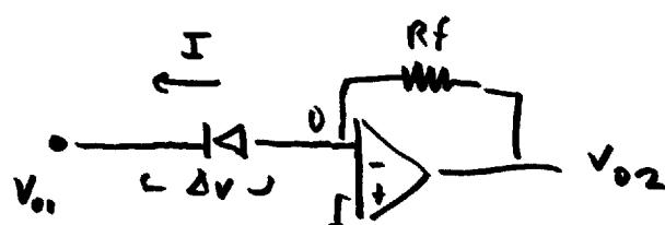
$$\Delta V = 0 - (+ V_i \times \frac{R_1}{R_1 + R_2} - V_T \ln \left( \frac{I_{ref}}{I_0} \right))$$
